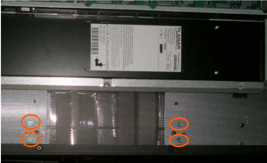
Landscape holes for kickstand bracket installation
